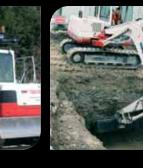
With 52.7kN bucket breakout force and 45kW rating, the TB175 provides a powerful operating ability.
