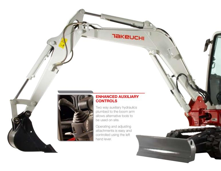
On site, the 3.5 tonne compact excavator is best known for reliable performance and regarded as a favourite by many operators for both comfort and control. Takeuchi achieve this with highly engineered reliable and touch sensitive controls.
