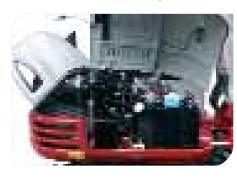
Side-by-side radiator and hydraulic oil cooler ensures fresh cool air reaches each cooler improving efficiency and component life. The A/C condenser is mounted on a hinged frame - decreasing inspection and cleaning time.
