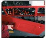
Removable floor and side panel for greater access to hydraulic control valve and piping.
