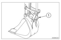
When lifting loads, install the sling on the lifting device (1).
