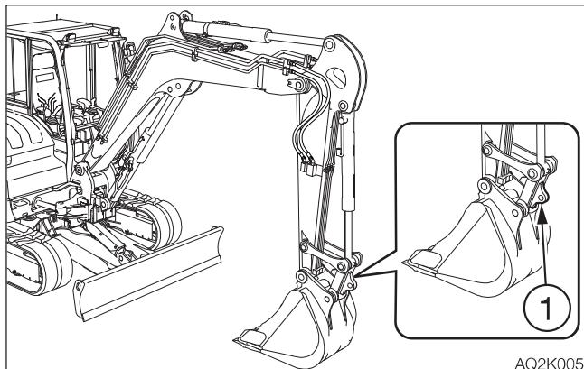
When lifting loads, install the sling on the lifting device (1).
